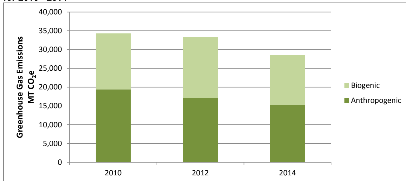
Figure 2: Comparison of the MWMC Facilities' Anthropogenic and Biogenic Emissions for 2010 - 2014
