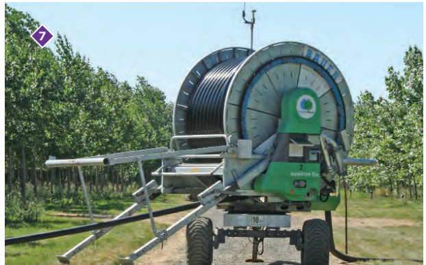
Recycled Water Irrigation Hose Reels
