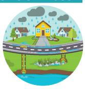
do not allow rain to soak into the ground. Underground pipes and catch basins, along with water quality facilities, are built to prevent flooding and filter pollutants from stormwater.
